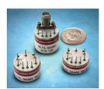
Two series of TO-8 oscillators, permanent magnet and electro magnetic are now available in production quantities. Extremely small size, excellent phase noise and good frequency stability make these oscillators the perfect choice for next generation, PXI, compact PCI, synthesizers and general applications. Units operate with low DC voltage and do not require a heater.
