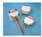
These electromagnetic tuned oscillators utilize a traditional magnetic structure to generate the required wide band frequency ranges over the 700 MHz to 8 GHz band. PC Board, PCI, PXI, VME & VXI sizes (1" x 1" x .5") are also available in these oscillator series. Excellent phase noise performance is offered over the 3-6 GHz band of -130 dBc/Hz at 100 kHz offset. Commercial and extended temperature range models are available throughout the product line.
