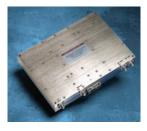
These frequency synthesizers covering wideband frequencies in the 600 MHz to 16 GHz band, out perform most test equipment signal generators available today. Extremely low phase performance over .6-3 GHz, 2-8 GHz, 2-10 GHz, and 6-13 GHz is available as standard products. Units utilize a 10 MHz external reference and provide 1 Hz frequency resolution. +10 to +12 dBm RF power output levels are provided.
