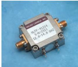
Utilizing the same small packages as the MLFI Series, these narrow band filters tune over a 2 to 3 GHz range. 50 MHz minimum 3 dB bandwidths are offered as standard. With no heater required, these filters are a good choice where low power consumption is required. The size of these filters is ideal for VXI, VME and the new PXI and PCI applications. Commercial and extended temperature ranges are available as special order.
