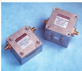
Industry standard 1" cube, 1.2" low profile, 1.4" cube, 1.7" cube and 2" cube package styles are offered. Tuning bands in the octave, multi-octave and ultra wide band configurations are standard throughout the product line. 2, 4, 6, 7 and 8 stage designs are available providing from 45 dB to over 120 dB rejection. Dual Channel, Low Ripple and Millimeter Wave configurations make these standard filter designs the largest filter offering on the Market today.
