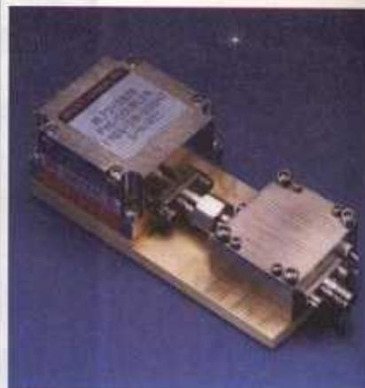
The MLPX models consist of a fundamental oscillator and a frequency doubler.
