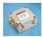
New series of Band Reject (Notch) Filters are now available with superior notch depths and bandwidths. Octave and multi-octave bands are offered over the 350 MHz to 20 GHz frequency range. Standard 1.7" or 1.7" low profile packages with SMA connectors are provided. Notch depths of 50 dB to 60 dB are available with up to 24 stages provided in some models.
