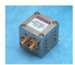
Band Reject (Notch) filters are offered covering the 2 to 20 GHz frequency range. Octave, multi-octave and full band designs are available as standard products. All designs are offered in a 1.4" cube standard package with SMA connectors. Precise notch depths of 40 dB are offered with up to 16 stages in some models available.
