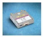
Frequency ranges of .6-2.5 GHz, 2-8 GHz, 6-13 GHz, and 8-16 GHz are standard in the product family. Special frequency ranges can be specified by the user. Units can be provided with internal, external or both crystal oscillator references. 1 KHz frequency resolution is standard. Fullband tuning speeds of 5-6ms are standard. +10 to +13 dBm power levels are provided depending on frequency. Control is via 5 line SPI or standard USB. Size is 2.5" x 2.5" x either .50" or .65" tall.
