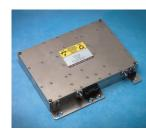
These narrow band synthesizers covering 2 GHz and 3 GHz tuning ranges over the 2-16 GHz frequency range, provide excellent phase noise performance for those difficult frequency converter designs. Units provide 1 Hz frequency resolution while using an industry standard 10 MHz reference input. +13 dBm to +10 dBm is provided depending on frequency band.
