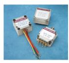
These electromagnetic tuned oscillators utilize a traditional magnetic structure to generate the required wide band frequency ranges over the 700 MHz to 10 GHz band. PC Board, PCI, PXI, VME & VXI sizes (1" x 1" x .5") are also available in these oscillator series. Excellent phase noise performance is offered over the 3-6 GHz band of -130 dBc/Hz at 100 kHz offset. Commercial and extended temperature range models are available throughout the product line.
